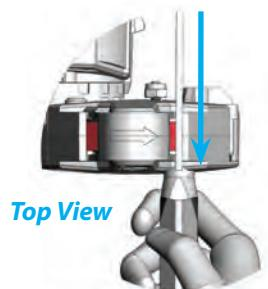
**Note:** proper knife-sharpening position; blade against outer edge of guide. Place knife blade in the guide so that the side of blade is firmly against the outside edge of the guide slot. Insert knife blade all the way to the bolster / finger guard.
